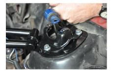
Step Four: Install the shocks using the four  $5/16 \times \frac{3}{4}$  flange bolts supplied with the export brace and tighten down.
