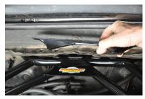
Install four 3/8 x 16 x 1 flange bolts through the
