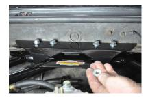
Step Three: Install the shock mounts on top of the export brace.
