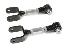
Adjust the length of the arm by placing a wrench on the adjusting hex sleeve. This is approximately two inches long located between the jam nuts. Rotating the adjuster will change the length of the arm. **DO NOT** adjust one end of the arm by itself! Use the adjuster. Adjusting one end only will offset the amount of threads required for holding the arm together when installed on the car.
