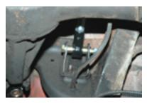
4. Check pinion angle: The pinion angle should be set with the vehicle at ride height on a drive on ramp. Measure the angle between the rear end and drive shaft. We recommend 2 to 3 degrees nose down. To adjust the angle, simply adjust the length of the upper control arm by using a one-inch wrench. Loosen the
