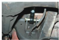
5. Check pinion angle: The pinion angle should be set with the vehicle at ride height on a drive on ramp. Measure the angle between the rear end and drive shaft. We recommend 2 to 3 degrees nose down. To adjust the angle, simply adjust the length of the upper control arm by using a one-inch wrench. Loosen the jam nuts first and then rotate the hex adjuster, by lengthening or shortening the upper arm will adjust the pinion angle. After the pinion angle is
