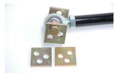
passenger. You should be reading number six. The plate on the forward side of the bracket should have hole 6 against the bracket.
