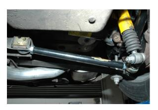
10. Follow the same procedure for the other side. Once both sides are complete you will require a rear wheel alignment. The alignment is handled by loosening the jam nuts on the strut rod and turning the strut rod. Once the alignment is achieved tighten down the jam nuts locking the strut rod in place.
