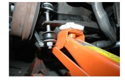
You will leave the floor jack in place till you have completed installing the new kit.
