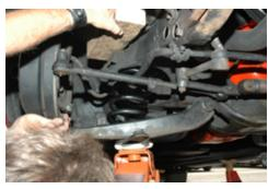
6.Raise the upper arm and spindle assembly up and slide a 2x4 up between the frame and upper arm. This will hold the assembly out of the way so you can work on the lower.
