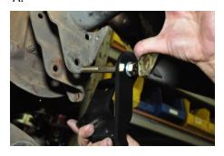
C. Install one  $\frac{1}{2}$  x 20 x 1-1/4 bolts with a 12mm flat washer through the hole that is aligned with the original shock mount hole. Tighten down the bolt to 70 foot pounds.
