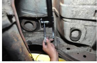
Once the cross member is lined up tighten down the shock mount bolts.
