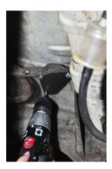
3. Install the shock mount brackets, remove the drill template and locate one of the shock mounts. There is a right and left mount. The mounts only install one way. Using the new hardware supplied, bolt the mount to the frame. Use one  $5/16 \times 18 \times 34$  bolt and one 5/16 whiz nut in the single hole towards the rear
