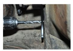
Depending on the frame you may have to use a shim between the frame and the new cross member. We have supplied one for each side. The shim would go between the bracket and the frame - see photo below. Install the  $3/8 \times 24 \times 1-1/4$  bolts using a flat washer first through the cross member and then use a  $3/8 \times 24$  whiz lock nut. Tighten to 45 foot pounds.
