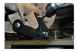
E. Install another  $\frac{1}{2}$  x 20 x 1  $\frac{1}{4}$  bolt with a 12mm flat washer on each side and torque to 70 foot pounds.
