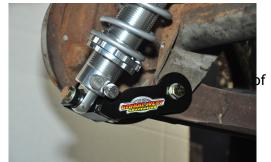
Adjusting the ride height is done by rotating the adjusting nut just below the spring. A spanner wrench included in your kit. The adjusting nut below the coil spring seat is a jam nut. The ride height is adjusted by turning the spring seat, Up raises the car and down lowers the car. Adjusting the ride height is best done by raining the car by the frame and removing tension on the spring and shock. After setting your desired ride height run the jam nut up to the spring seat and tighten.
