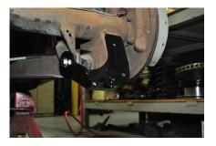
C. Install one  $\frac{1}{2}$  x 20 x 1-1/4 bolts with a 12mm flat washer through the hole that is aligned with the original shock mount hole. Tighten down the bolt to 70 foot pounds.
