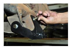
8. Install the shocks starting with the upper mount. Use a  $\frac{1}{2}$ inch x 20 x 3 ½ inch long bolt with a 12mm flat washer and slide it through the upper shock mount. Hold the shock in
