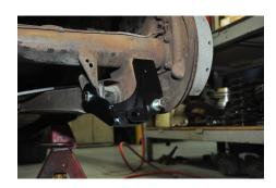
D. Use a drill with a  $\frac{1}{2}$  inch drill bit and drill a new hole through the differential lower arm mount.
