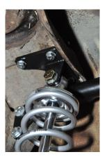
9. Install a  $\frac{1}{2}$  x 20 x 3  $\frac{1}{2}$  bolt with a 12mm flat washer through the lower shock mount. The adjusting knobs need to be on the positioned towards the inside of the car.
