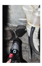
3. Install the shock mount brackets, remove the drill template and locate one of the shock mounts. There is a right and left mount. The mounts only install one way. Using the new hardware supplied, bolt the mount to the frame. Use one  $5/16 \times 18 \times 34$  bolt and one  $5/16 \times 18 \times 34$  bolt and one  $5/16 \times 18 \times 34$  bolt.
