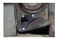
4. Time to install the cross member, slide the cross member up to the newly installed
