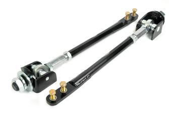
2. Install the assembled strut rod clevis up into the frame hole. The clevis will only install one way. The curved portion goes down allowing the face of the clevis to go flush against the frame. There is a gold ring around the bolt that is used to index the clevis in the frame.
