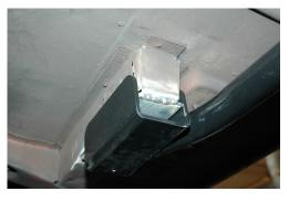
The back portion of the subframe will slide over the rear frame rail that goes over the differential.
