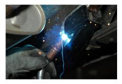
Note: Do not weld along the top of the forward boxes of the subframe. It is not required. If you choose to do so, you will need to remove the carpet inside the car.
