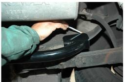
2. Use a dead blow hammer and tap the 911 into place. The 911 should be as tight to the floor as possible. If the subframe doesn't stay in position, a clamp will work nicely or get someone to help hold it up to the floor so you can mark the location of where the subframe will require welding.
