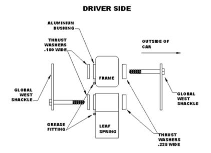
Using the  $\frac{1}{2}$  inch bolts supplied in your kit, finish assembling the shackle. You can install the bolts from the inside or outside, it makes no difference. Hang the shackles of the frame first and then slide the leaf up into position. Install the locking nuts.
