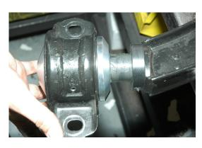
10.Install the grease fitting and you are ready to install the assembly on the car. Install
