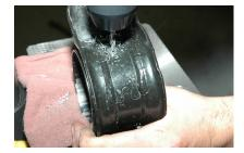
8. Time to press the big rear bushing into the bracket. Align the side hole in the bushing with the grease fitting hole in the bracket. Place the assembly into the press and press the bushing into the bracket till the lip of the bushing contacts the bracket.
