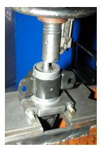
Once the bushing with the bracket is press off the arm you will need to get the bushing out of the bracket. - You first must buff off the flange on the bushing so you can get a fixture to index directly on the bracket.
