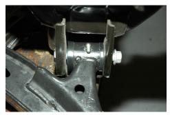
Do not pry the rear bushing bracket over in an attempt to gain more caster. You will put the bushings in bind and induce drag.
