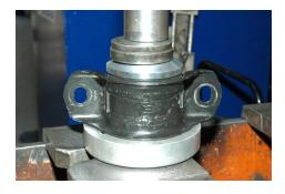
9. Next take the Blackline bushing insert and lubricate the inside of the bushing and the bushing housing. Slide the insert onto the lower control arm pin. The bushing should move freely. Next slide the housing over the insert.
