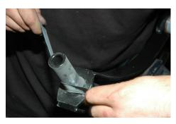
5. Drill a grease fitting hole in the front bushing housing on the top of the arm (ball joint pointing up). You are going to drill a #3 hole (.210) in the center. The arm is laying flat on the table. Go straight down. Once the hole is installed, use a ¼ x 28 tap and tap the hole. Clean the hole from having any burrs. A 90 degree grease fitting is furnished in the kit. Install the grease fitting so the fitting points towards the ball joint.
