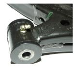
7. Next you must drill a hole in the rear big bushing bracket for a grease fitting. The hole must be placed around 40 to 45 degrees from the bolt hole pointing to
