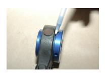
6. Once the press work is complete, lubricate the inside of the white insert with grease. We recommend using synthetic grease that is water resistant.
