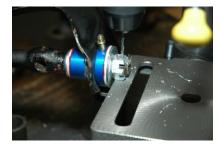
12. Install a cotter pin after drilling.
