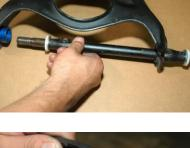
11. Use a 1/8-inch drill bit and drill a 1/8-inch hole through the shaft. You are going to cotter pin the hex nut so there will be no chance of the nut backing off. The hole should be drilled in the slot of the hex nut similar to that of a wheel bearing cotter pin setup. Cotter pin each end of the shaft before installing on the car.
